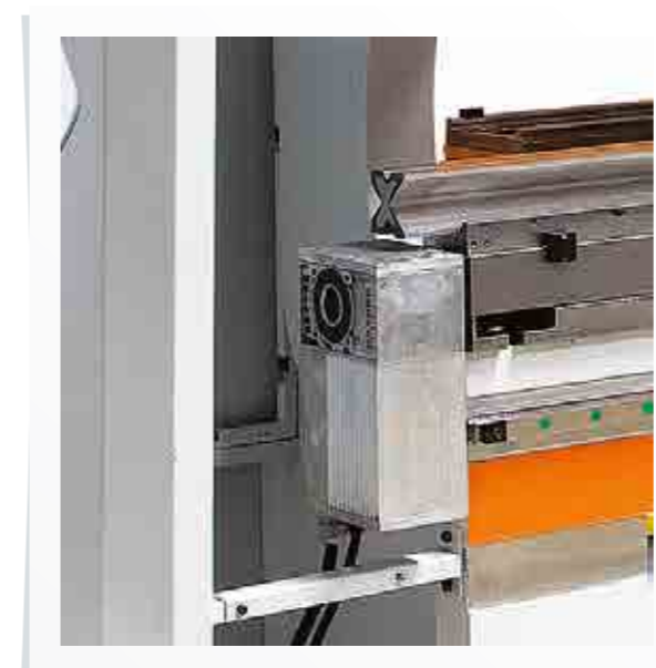
CNC Motorised Crowning System (S) CNC crowning system that communicates with the CNC controller, performs crowning automatically and enables the part to be at even bending angle at any given point.
