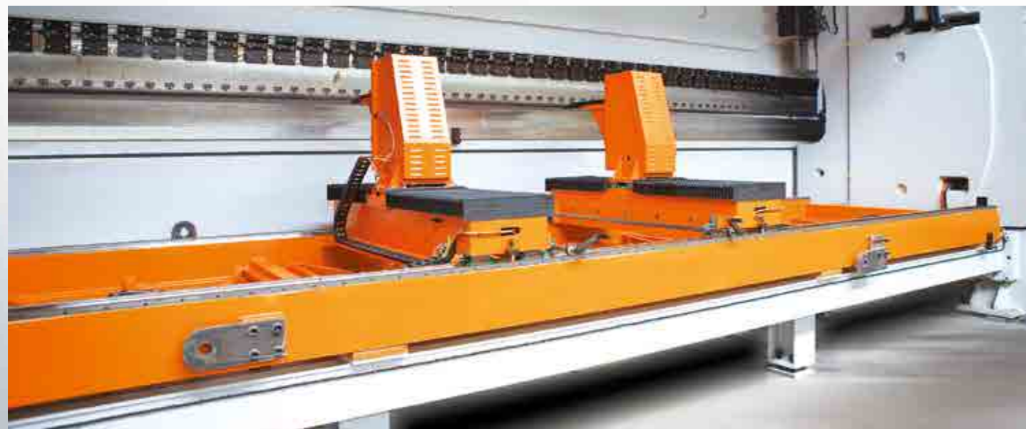
Heavy type 6 axes (Y 1 , Y 2 , X 1 , X 2 , R 1 , R 2 ) servo motorized back gauge.
