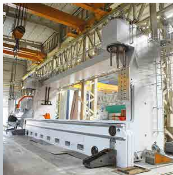
Speed-Bend 14800 x 1500 TN production line.
